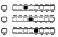
**SCRATCH HOLD** – This effect works like the above except the music will not release when the wheel is pushed forward. It is basically the same as scratching on a powered off turntable. *Scratch is similar to working with a playing turntable, while the Scratch hold is similar to scratching a turntable with the power off.*
